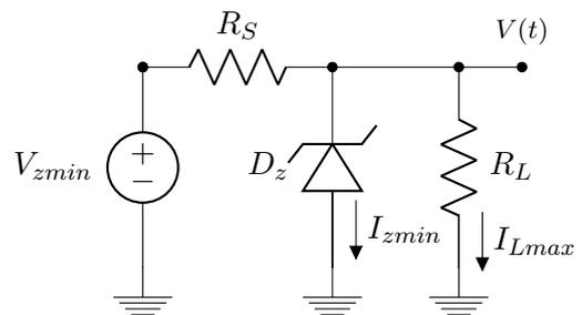
$$\frac{13.3 - 6.2}{R_S} = I_{Zmin} + I_{Lmax} = 30 \times 10^{-3}$$
