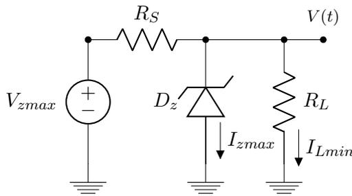
$$\frac{18.9 - 6.2}{R_S} = I_{Zmax} + I_{Lmin} = 70 \times 10^{-3}$$
