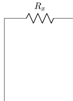
Onde  $R_x = R_1 + R_2 + R_3$ .
