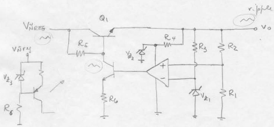
$$V_o = \left( 1 + \frac{R_2}{R_1} \right) V_{z1}$$
