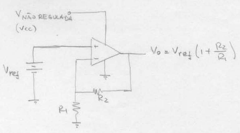
$$V_o = V_{ref} \left( 1 + \frac{R_2}{R_1} \right)$$
