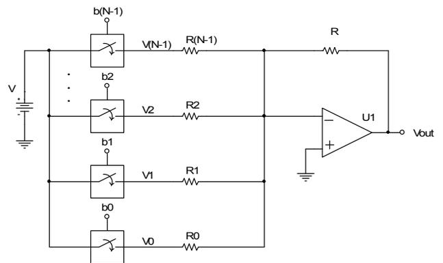
$$V_{out} = -\left( \frac{R}{2^N R} b_0 + \frac{R}{2^{(N-1)} R} b_1 + \frac{R}{2^{(N-2)} R} b_2 + \dots + \frac{R}{2^1 R} b_{(N-1)} \right) V$$
