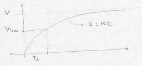
$$V_{lim} = 2 V_{om} \frac{R_2}{R_1 + R_2}$$
