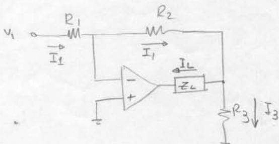
$$I_L = I_1 - I_3 = \frac{V_1}{R_1} - \frac{V_1 \left( \frac{R_2}{R_1} \right)}{R_3} = -\frac{1}{R_3} \frac{R_2}{R_1} V_1$$
