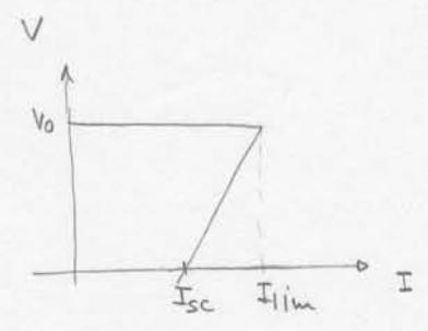
$$(V_o + I_{lim} R_{sc}) \frac{R_x}{R_x + R_y} + V_{BEQ_2} = I_{lim} R_{sc}$$
