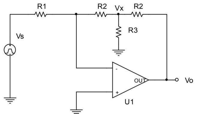
$$V_x = \frac{V_o}{\left(2 + \frac{R_2}{R_3}\right)}$$
