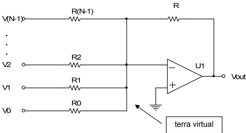
$$V_{out} = -\left( \frac{R}{R_0} V_0 + \frac{R}{R_1} V_1 + \frac{R}{R_2} V_2 + \dots + \frac{R}{R_{(N-1)}} V_{(N-1)} \right)$$
