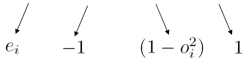
$$\frac{\partial J}{\partial w_{ij}} = \frac{\partial J}{\partial e_i} \frac{\partial e_i}{\partial o_i} \frac{\partial o_i}{\partial u_i} \frac{\partial u_i}{\partial w_{ij}} = -e_i(1 - o_i^2)x_j$$
