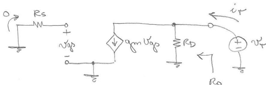
$$\text{Como } V_{gp} = 0 \text{ nesse circuito: } i_T = \frac{V_t}{R_D} + \alpha_m V_{gp}$$
