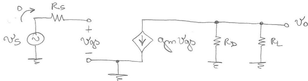
$$V_0 = -\alpha_m V_{gp} \cdot R_D // R_L = -\alpha_m V_S \cdot R_D // R_L$$
