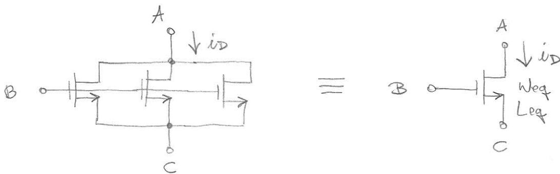
$$k_n \left( \frac{W_1}{L_1} + \frac{W_2}{L_2} + \frac{W_3}{L_3} \right) \left[ (V_{GS} - V_{th}) V_{DS} - \frac{V_{DS}^2}{2} \right] = k_n \frac{W_{eq}}{L_{eq}} \left[ (V_{GS} - V_{th}) V_{DS} - \frac{V_{DS}^2}{2} \right]$$
