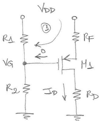
$$V_G = \frac{R_2}{R_1 + R_2} V_{DD} = \frac{160}{40 + 160} \cdot 10 = 8,0 \text{ V}$$
