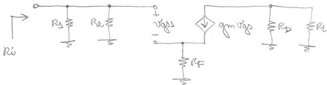
$$R_i = R_1 // R_2 = 32 \text{ k}\Omega$$
