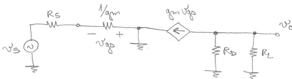
$$v_{gs} = - \frac{1/gm}{R_s + 1/gm} \cdot v_s \quad \rightarrow \quad v_o = - gm v_{gs} \cdot R_D // R_L$$
